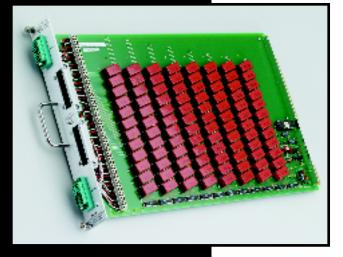
The Model 7071 General Purpose Matrix Card is an 8×12 configuration that switches High, Low, and Guard at each of the 96 relay crosspoints. The eight rows are connected automatically to the general purpose analog backplane when the matrix card is installed into the 707A and 708A mainframe. This allows for easy expansion in 12 column increments and eliminates the requirement for wiring between cards.
